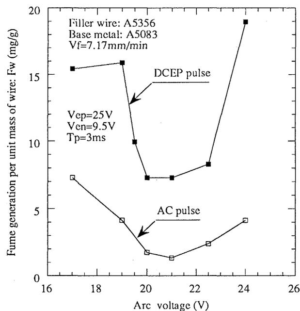
Fig.7 Effect of welding voltage on fume generation
