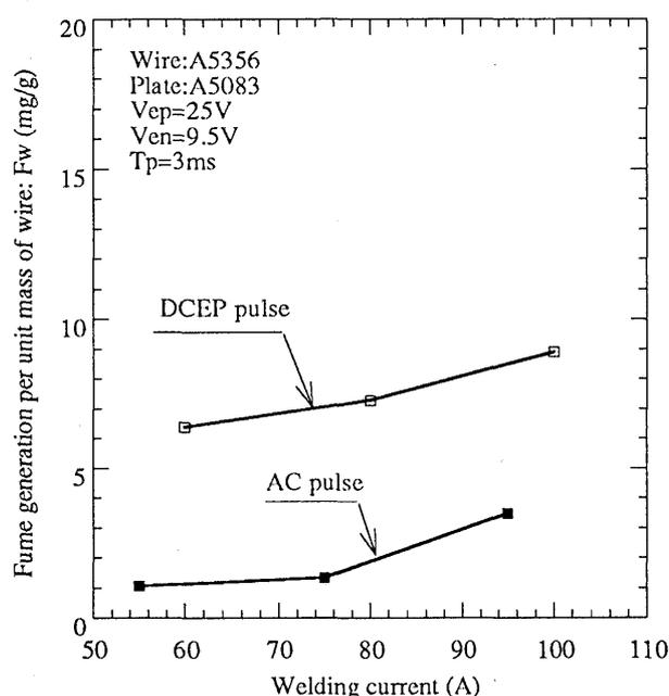
Fig.6 Effect of welding current on fume generation
