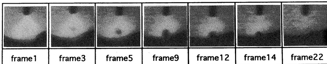
Fig.9 Droplet transfer of AC-pulsed GMA welding
