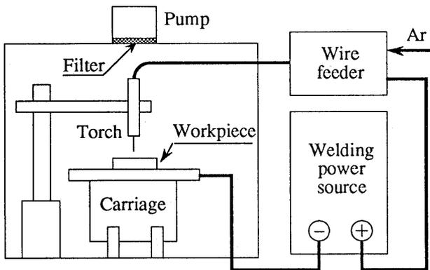
**Fig.4** Schematic diagram of weld fumes collection set-up
