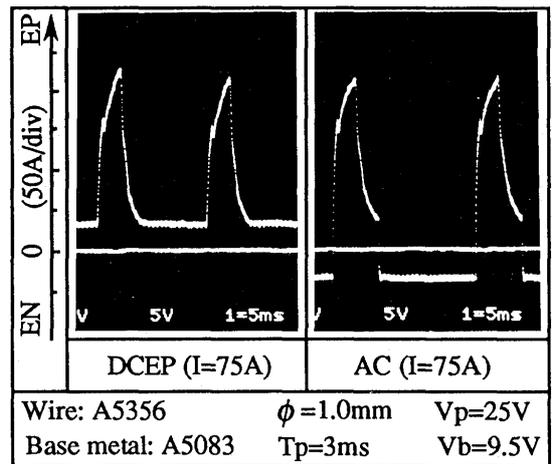
Fig.3 Current waveform of DCEP and AC pulse
