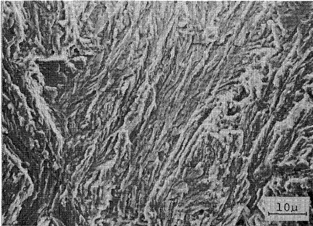
(a) cleavage-like fractured surface
