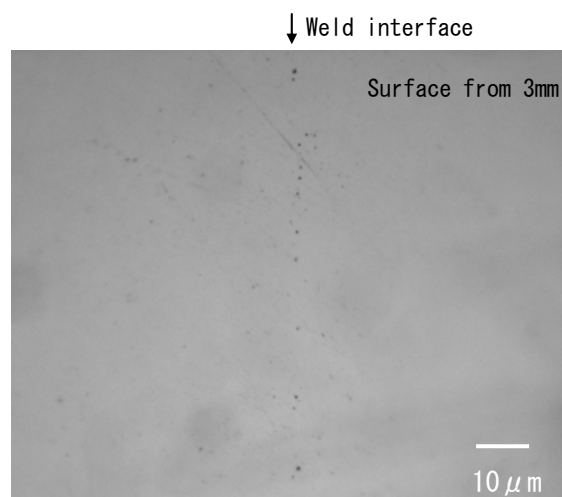
Fig.4-15 The state of oxide inclusions on cross-section (5) : TPN0.R-2
