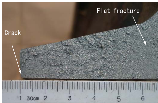
Fig.5-7 The appearance of fracture surface (TPNo.2-2)
