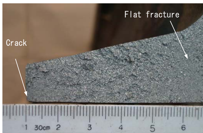
Fig.5-7 The appearance of fracture surface (TPNo.2-2)
