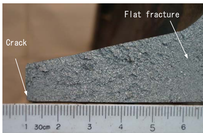
Fig.5-7 The appearance of fracture surface (TPNo.2-2)
