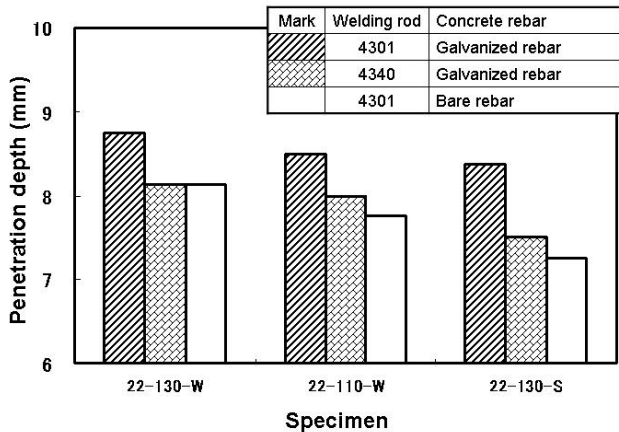
Fig. 4 Influence of different parameters on penetration depths of flare joints.
