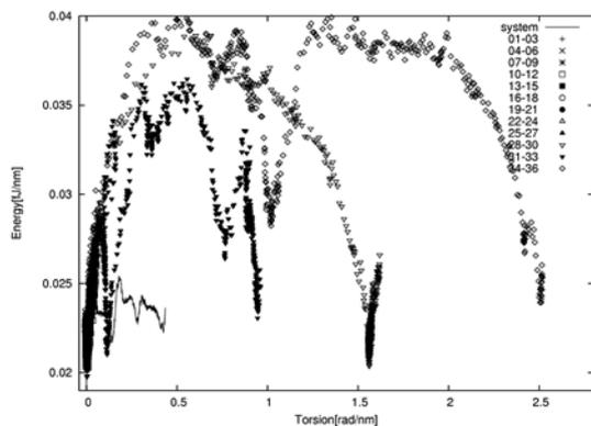
**Fig. 5** Potential energy vs torsion angle.
