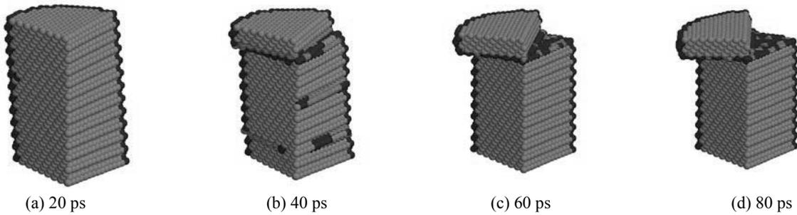
**Fig. 3** Atomic arrangement of quarter Cu nanowire under  $\langle 111 \rangle$  torsion
