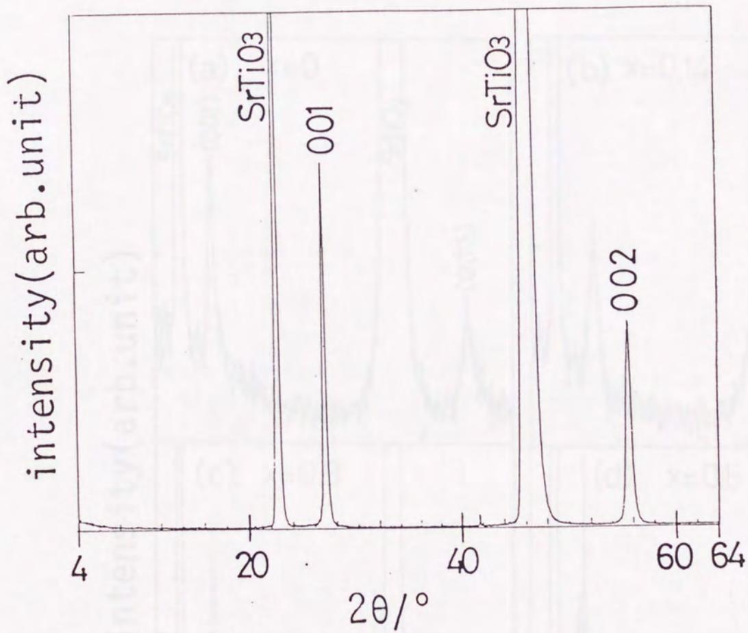
Fig.6 X-ray diffraction pattern of as-grown  $\text{Ca}_{0.86}\text{Sr}_{0.14}\text{CuO}_2$  film.
