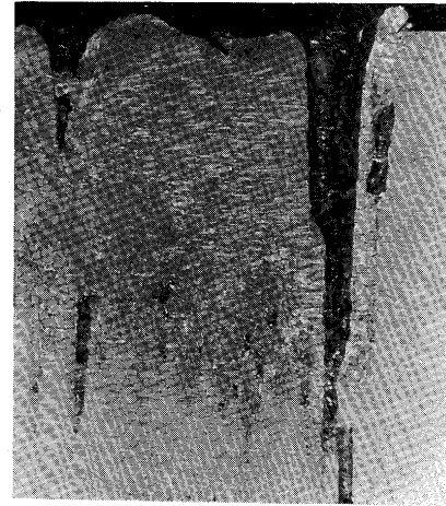
Aluminium (2S) 150 KV, 35 mA, 200 mm/min.
