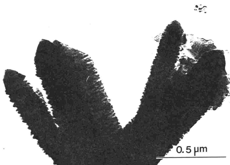
Figure 1-12. Transmission electron micrographs of incipient crystals washed in 1N-KOH solution.
