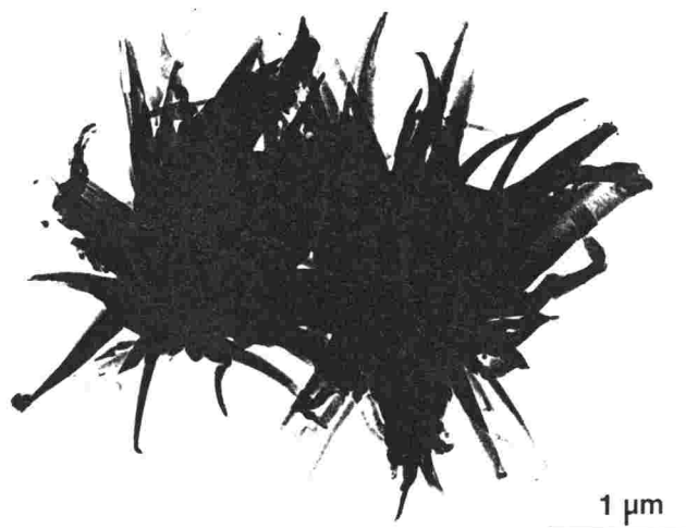
Figure 4-24. Transmission electron micrograph of incipient PMB whiskers prepared in LP at 300°C for 3min.
