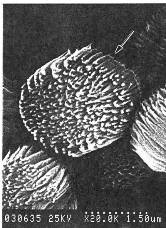
Figure 4-10. Scanning electron micrograph of POBP crystals prepared in TS 800 at 330°C for 4h.
