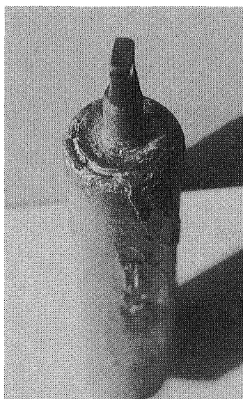
Fig. 5 Leakage occurred on welding part of W crucible
