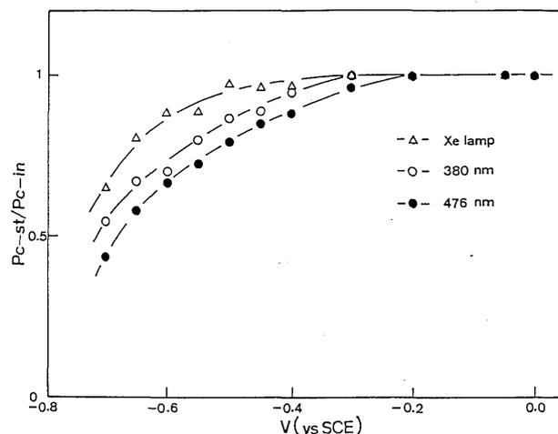
Fig. 7 Potential dependence of the transient ratio, (Pc-st/Pc-in) for photoresponse obtained with the polychromatic light of 300 W Xe lamp, 380 nm and 476 nm in 1% Y<sub>2</sub>O<sub>3</sub>-TiO<sub>2</sub> coatings produced by plasma gas Ar/H<sub>2</sub> in air and heat-treated at 400°C during 90 minutes.
