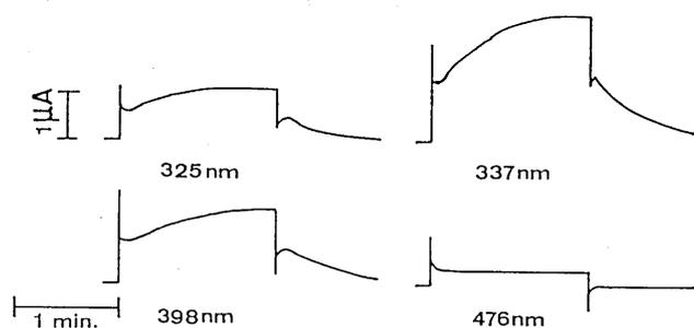
Fig. 8 Time dependence of the photocurrent and decays for various light wavelength in plasma sprayed TiO<sub>2</sub> coatings produced by TiO<sub>2</sub> powders (Nihon Abrasin Ltd).
