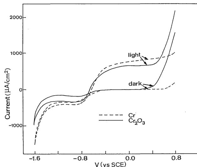
Fig. 5 Current-potential curves for plasma sprayed 1% Cr<sub>2</sub>O<sub>3</sub> and 0.5% Cr-TiO<sub>2</sub> coatings produced by plasma gas Ar in air.
