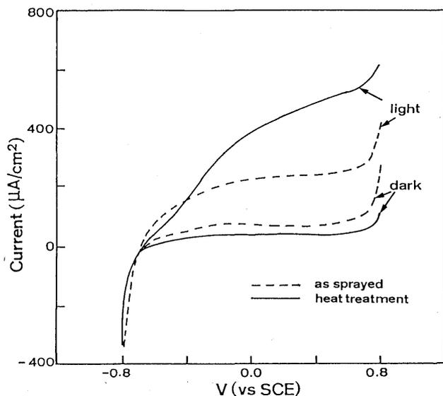
Fig. 3 Current-potential curves for plasma sprayed TiO<sub>2</sub> coatings produced by plasma gas Ar/H<sub>2</sub> in air and heat-treated at 400°C during 90 minutes.
