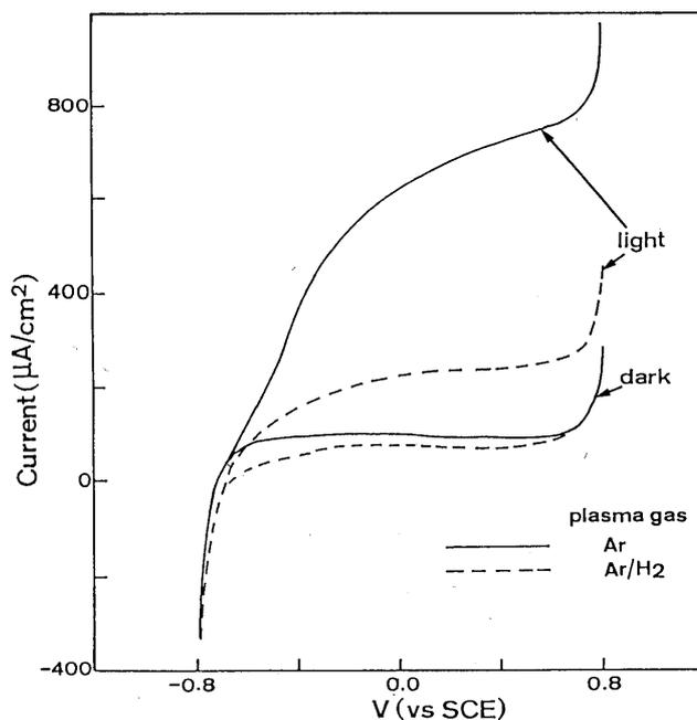
**Fig. 2** Current-potential curves for plasma sprayed  $\text{TiO}_2$  coatings produced by plasma gas Ar and  $\text{Ar}/\text{H}_2$  in air.
