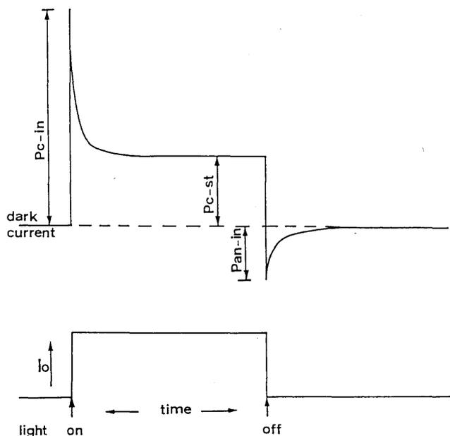
Fig. 6 Typical transient photoresponse of plasma sprayed TiO<sub>2</sub> coatings.
