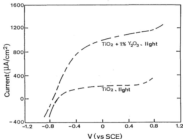
Fig. 4 Current-potential curves for plasma sprayed TiO<sub>2</sub> and 1% Y<sub>2</sub>O<sub>3</sub>-TiO<sub>2</sub> coatings produced by plasma gas Ar/H<sub>2</sub> in air and heat-treated at 400°C during 90 minutes.
