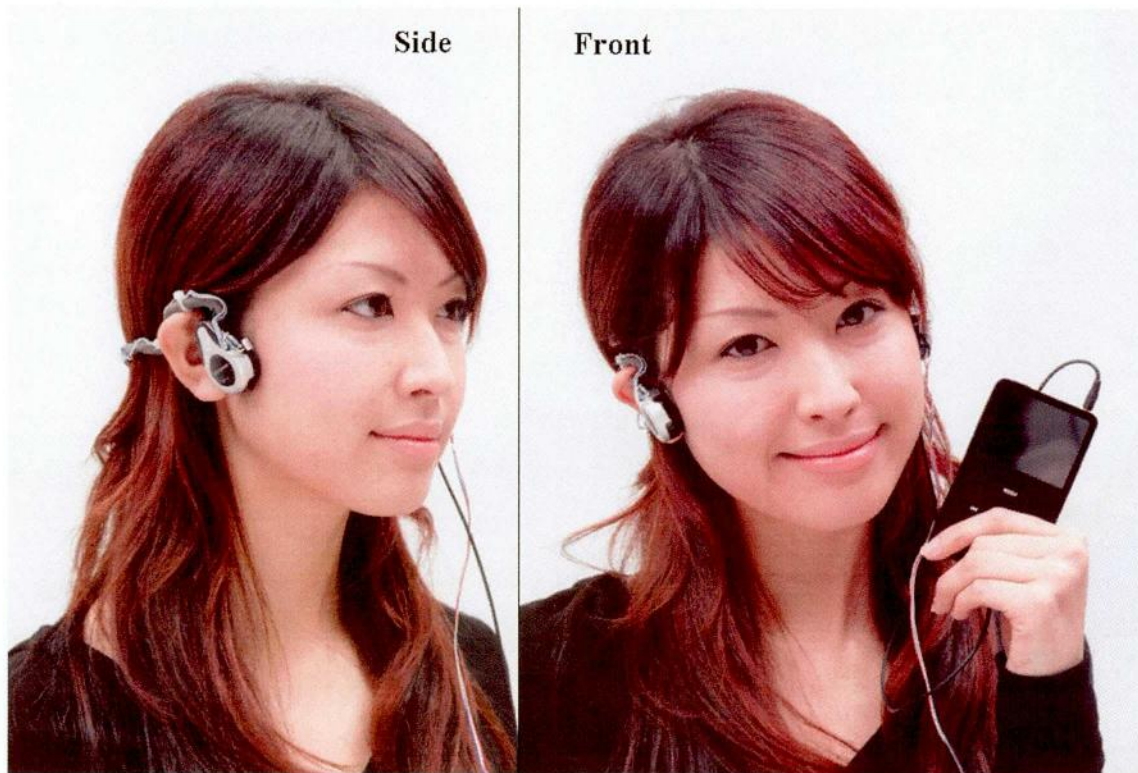
Fig. 2.45 Installation image of the KOMEKAMI switch
