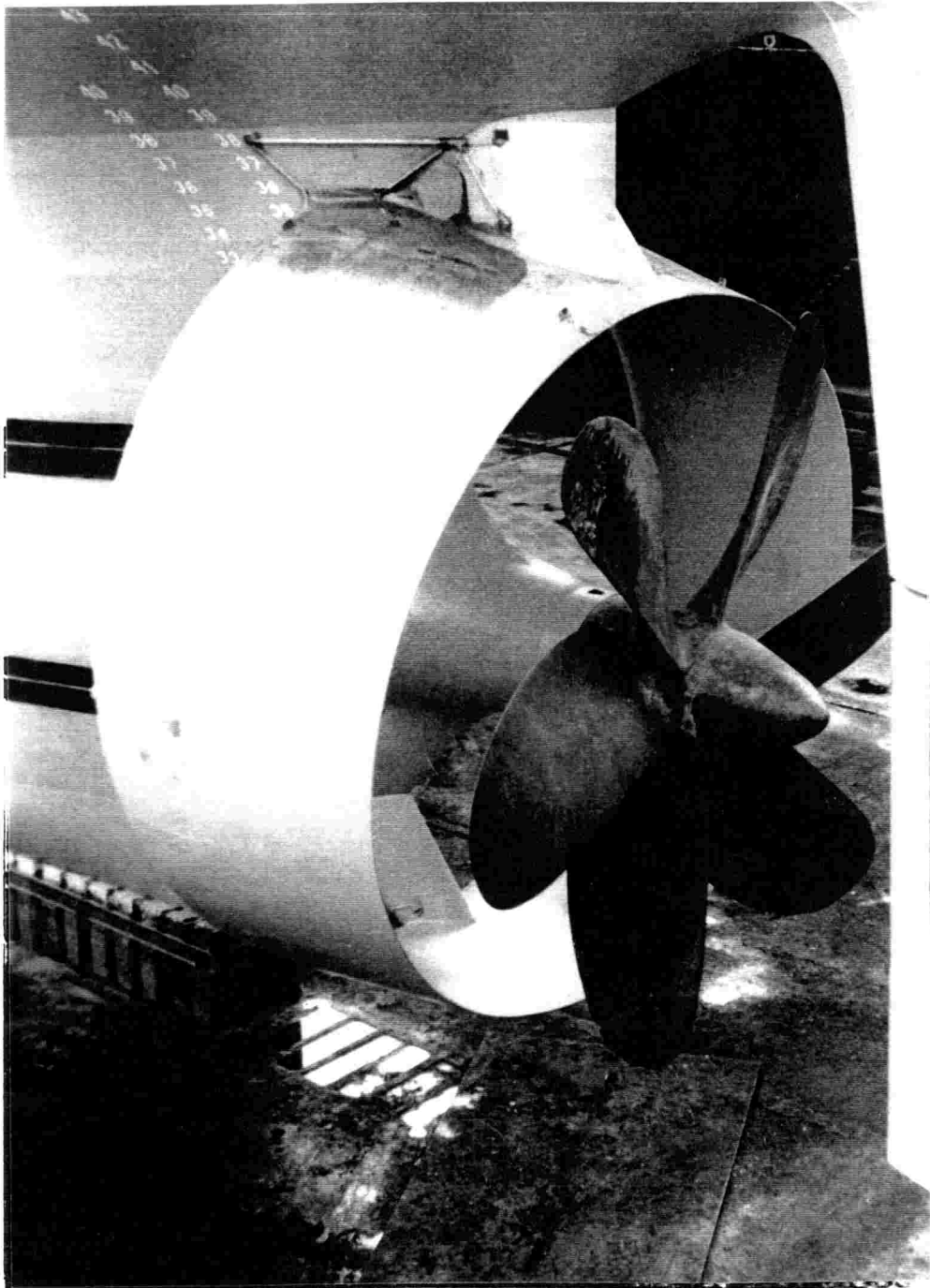
Fig. 2-14 Photo of MIDP Installation
