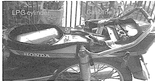
Fig. 12: Installation of LPG cylinder and gasoline tank on Honda Dream II LPG/gasoline bifuel motorcycle
