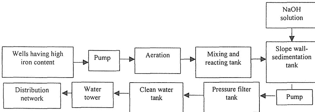
This technology was applied in Phuoc Kien (Nha Be district) with iron content varied from 57 to 65 mg/L, and in Hung Long (Binh Chanh district) with iron content varied from 85 to 105 mg/L. Both has very good treatment effect and stable operating till now (near two years).
