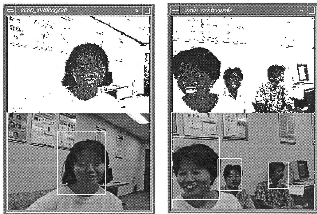
(b) Extracted faces candidate in live video sequence. The upper part shows the extracted region of the skin color and the hair color. The lower part shows the face detection result.
