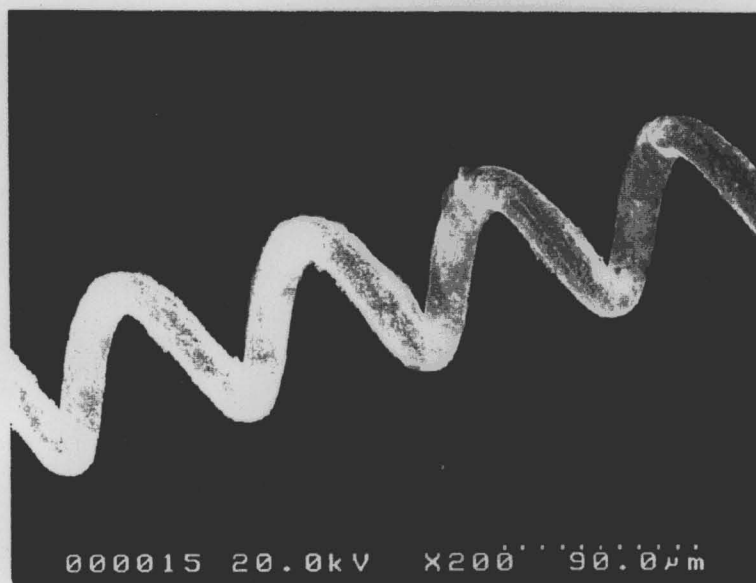
Fig.4.2 Coil type heating element for high temperature in-situ electron microscopy.
