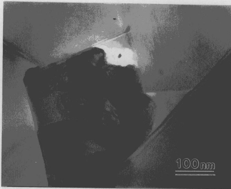
Fig.6.13 TEM image of nickel silicide agglomerate in the composite sintered at 1600°C.
