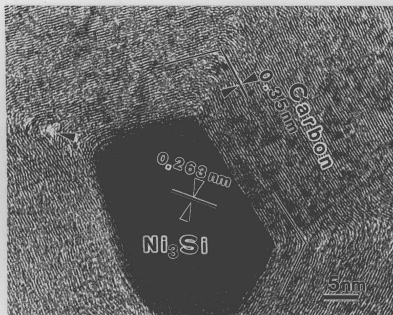
Fig.6.15 High resolution TEM image of the \text{Ni}_3\text{Si} nanocrystal encapsulated within carbon cage.
