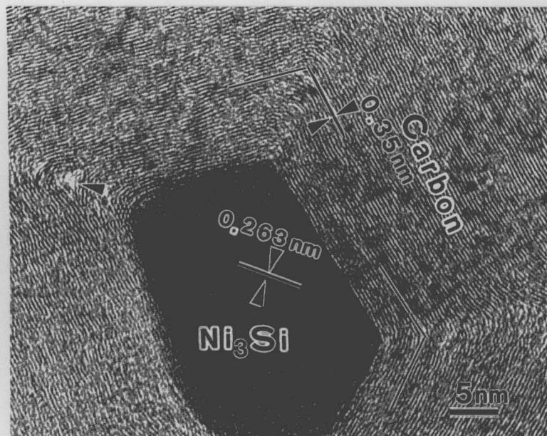
Fig.6.15 High resolution TEM image of the  $\text{Ni}_3\text{Si}$  nanocrystal encapsulated within carbon cage.
