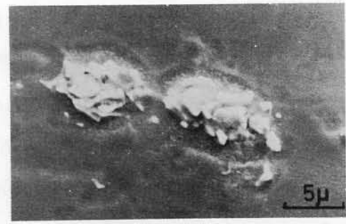
Fig.4-8 Scanning Electron Micrograph in Heat Affected Zone of Inconel 625 Electron Beam Welds
