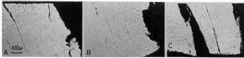
Fig.7-32 Microstructure of TIG Weld Joint Specimen of Hastelloy X (HAEM) Ruptured, at Weld Metal
