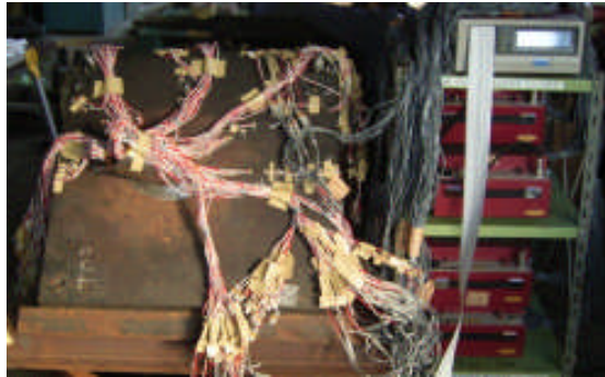
(a) Strain gauges and leads attached at inner and outer surfaces of the specimen
