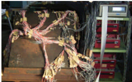
(a) Strain gauges and leads attached at inner and outer surfaces of the specimen
