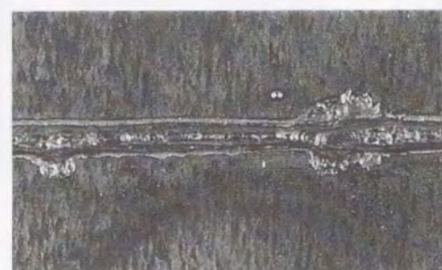
(a) Appearance of spot defect 5 mm
