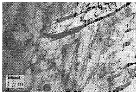
Fig 2-14 Transmission electron micrographs of ICCGHAZ subjected to 600°C third thermal cycle: (a) bright field image, (b) diffraction pattern and (c) its schematic representation (Tp 1 =1400°C、Tp 2 =750°C、Tp 3 =600°C)
