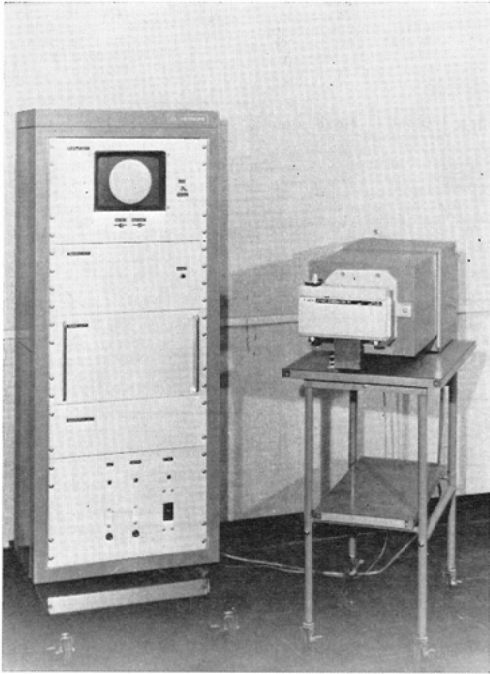
Fig. 12. Video disk memory unit and the display unit (left). Monitor flash unit (right).
