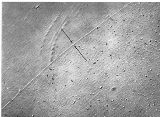
Fig. 3 Fission track (small specks) and  $\alpha$  track (fine dots) etch pits in a cellulose triacetate sheet. Arrows indicate a boundary line dividing the coated area (the lower right part) and the non-coated area (the upper left part)
