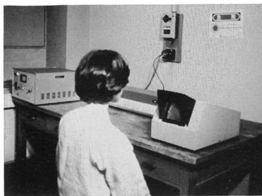
Fig. 4 Viewer for the Holographic Stereosynthesis
