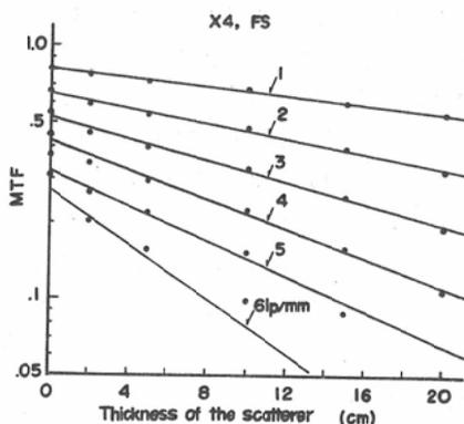
Fig. 3 Semi-logarithmic plots of MTFs of the scattered radiation for four-fold magnification according to thickness of the water phantom(cm) as a scatterer, when the spatial frequency is kept constant. Each line is normalized to the MTF value when the scatterer is not added.
