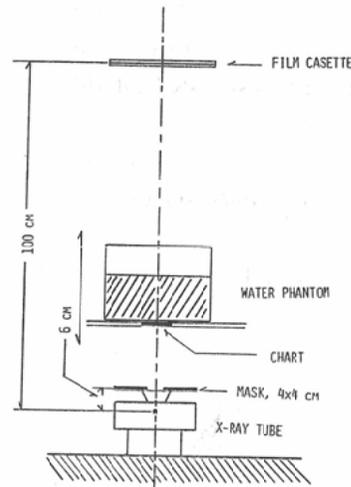
Fig. 1 Geometrical arrangement of the experimental devices.
