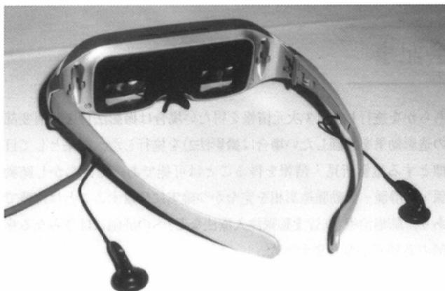
Fig. 1 Personal monitor (Sony Co. Glasstron Lite, PLM-A35)
