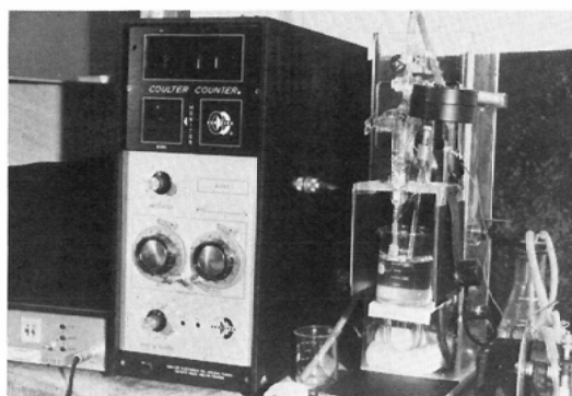
Fig. 1 Coulter Counter ZB-type Electronic counter (left) and sample stand (right)
