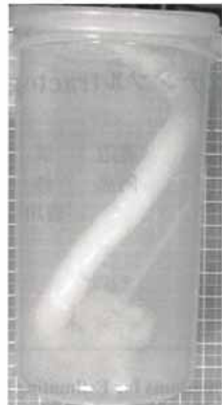
Fig. 2 Phantom of bundled polyester yarn (spirally twisted).
