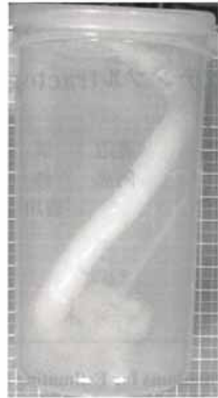
Fig. 2 Phantom of bundled polyester yarn (spirally twisted).
