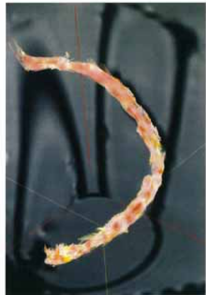
Fig. 4 Tractography of the polyester yarn phantom (spirally twisted).
