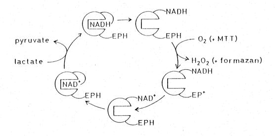
Fig. III-1. Schematic representation of the catalytic cycle of semisynthetic lactate oxidase. Only the cycle with the more reduced forms of  $\mathrm{EP}^+\mathrm{-LDH-NAD}^+$  is shown.
