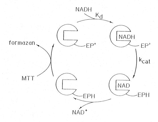
Fig. I-1. Schematic representation of the catalytic cycles of NADH oxidation by semisynthetic NADH oxidase.  $K_{\rm d}$ , the dissociation constant of the binding-site NADH complex;  $k_{\rm cat}$ , the turnover number of the active site.
