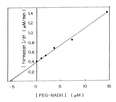
Fig. III-6. Effects of exogenous PEG-NADH on the activity of semisynthetic lactate oxidase. Lactate oxidase activity was measured by the MTT method. The reaction mixture contained the same components as described in the legend to Fig. III-5, except that PEG-NADH was added instead of 5-ethylphenazine; the initial concentration of PEG-NADH was varied and the values are shown on the abscissa.
