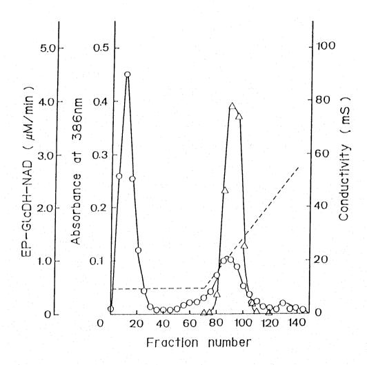
Fig. II-2. DEAE-Sephadex CL-6B column chromatography of EP<sup>+</sup>-GlcDH-NAD<sup>+</sup>. O , Absorbance at 386 nm;  $\Delta$ , EP<sup>+</sup>-GlcDH-NAD<sup>+</sup> activity; - - -, conductivity. The EP<sup>+</sup>-GlcDH-NAD<sup>+</sup> activity is expressed as glucose oxidase activity measured by the MTT method as described under "Experimental Procedures".
