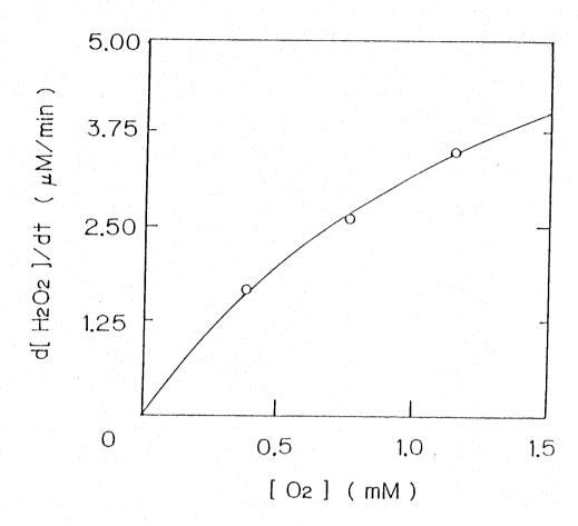
Fig. II-3. Effects of oxygen concentration on the activity of semisynthetic glucose oxidase. —, the activity calculated from the Michaelis-Menten equation with  $V_{max}=8.23~\mu\text{M/min}$  and  $K_{m}=1.57~m\text{M}$ .
