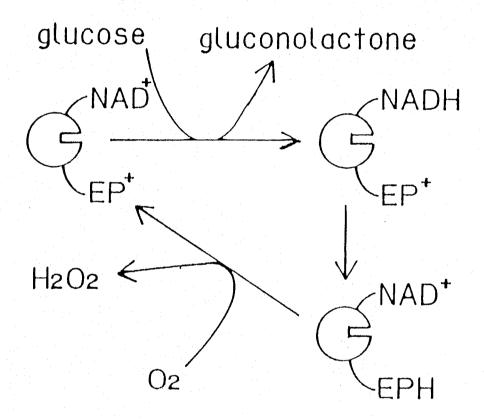
Fig. II-1. Schematic representation of the catalytic cycle of semisynthetic glucose oxidase. Only the cycle with the more oxidized forms of  $\mathrm{EP}^+\mathrm{-G1cDH-NAD}^+$  is shown.  $\mathrm{EP}^+$ , the oxidized form of the ethylphenazine moiety; EPH, the reduced form of the ethylphenazine moiety.
