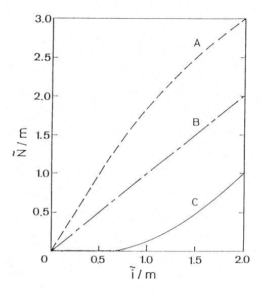
Fig. IV-4. Plot of i/m vs. N/m. The values of N/m were calculated using the following constants: K = 120, m = 4, n = 2, and  $\boldsymbol{\xi} = 2$  (for curve A), 1 (for curve B), or 0 (for curve C).
