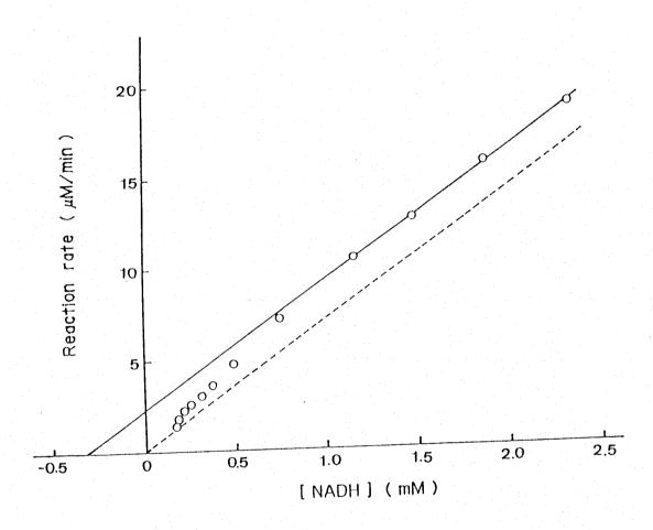
Fig. I-4. Effect of NADH concentration on the activity of EP<sup>+</sup>-PEG-G1tDH. The reaction mixture (3.2 ml) contained 1.73  $\mu$ M (as subunit concentration) EP<sup>+</sup>-PEG-G1tDH, 1.5 mM MTT, 0.1 M sodium phosphate (pH 7.5), and the indicated concentrations of NADH. - - -, theoretical line for the first term of Eqn I-10 with a klf value of 1.60 mM<sup>-1</sup>s<sup>-1</sup>.
