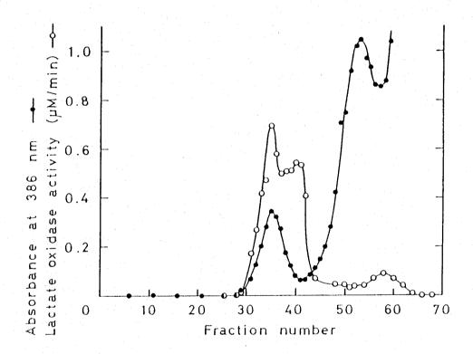
Fig. III-2. Sephacryl S-200 column chromatography of  $EP^{\dagger}$ -LDH-NAD $^{\dagger}$ .  $\bullet$ , absorbance at 386 nm; O, lactate oxidase activity. Lactate oxidase activity was measured by the MTT method as described under "Experimental Procedures"; reactions were started by adding 0.2 ml of sample solution to a substrate solution (3.0 ml) contained 0.1 M sodium phosphate, pH 7.5, 50 mM lithium L-lactate, and 1.5 mM MTT.
