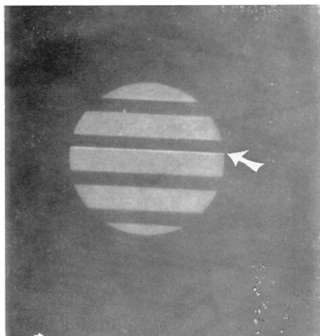
Fig. 3, Parallel X-ray beam position indication transmitted through copper and lucitepile.
