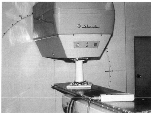
Fig. 2 Photograph showing electron beam irradiation equipment used in the present experiment.
