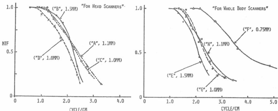
Fig. 5. Modulation transfer function of 8 scanners.
