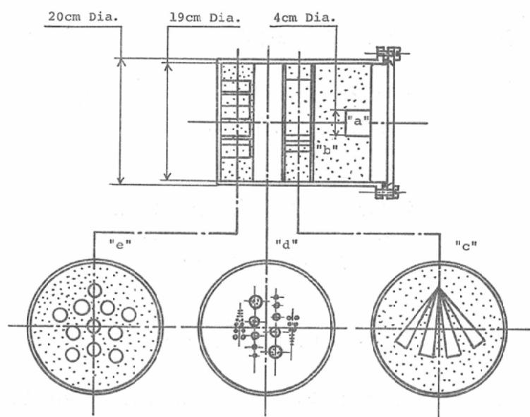
Fig. 1. Schematic representation of the phantom for performance evaluation. "a" ... Contrast scale, "b" ... Noise and contrast scale, "c" ... MTF, "d" ... Spatial resolution, "e" ... Contrast resolving power and linearity.
