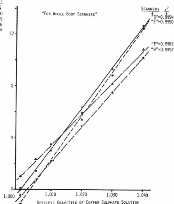
Fig. 4. CT number mean values against various specific gravities of copper sulphate solution (Linearity tests for 8 scanners).  $\gamma$ : correlation coefficient.
