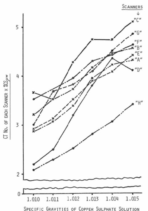
Fig. 3. Results of contrast resolution tests for 8 scanners.
