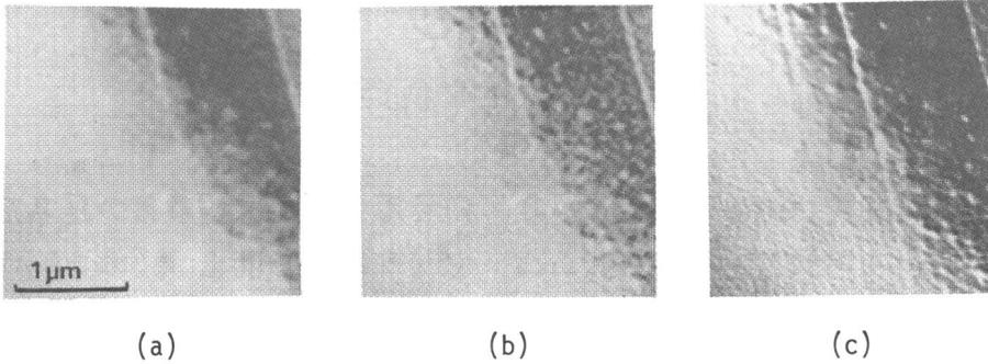
Fig. 43 Experimental results of contrast enhancement of an electron micrograph of copper taken by the HVEM (High-voltage Electron Microscope) at 2MV.
