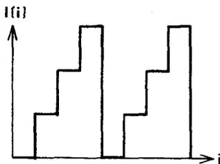
Fig. 48 Characteristic curve for MSB and 3LSB removal.
