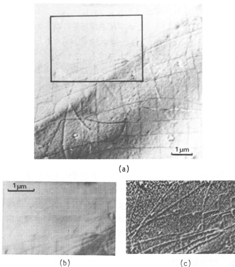
Fig. 45 Experimental result of contrast enhancement of a dislocation image by the nonlinear filtering.
