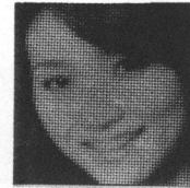
Fig. 11 Image displayed on the CRT monitor, which is detected by the 2-D 64 \times 64 image sensor.
