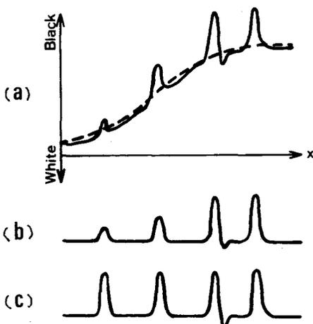
Fig. 44 Illustrating diagram of extraction of dislocation lines in a dislocation image under the variable background level.
