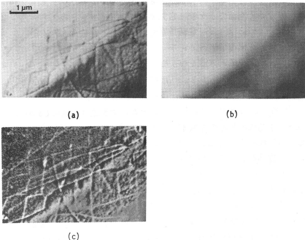
Fig. 60 Experimental results of extraction of dislocation lines from an electron micrograph of an aluminum by using the hybrid system.
