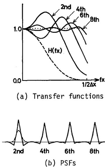
Fig. 26 Transfer functions and PSFs of a Gaussian blur system (broken line) and those for the systems restored by the Linear combinations of 2nd, 4th, 6th and 8th derivatives under the constraint of  $f_0 = 1$ , in which the transfer function of the desirable system (dot line) has unity all over entire spatial frequency region.
