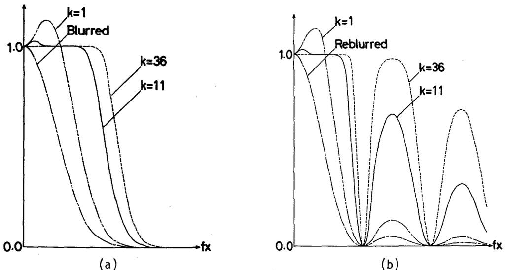
Fig. 52 Spatial frequency responses for the PSFs restored by the iterative restoration method on finite number ( $k=1, 11$  and  $36$ ) of iterations.
