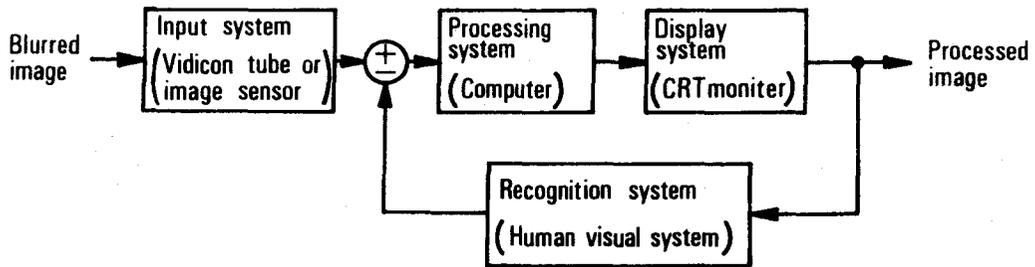
Fig. 1 Man-machine feedback looped image processing system.
