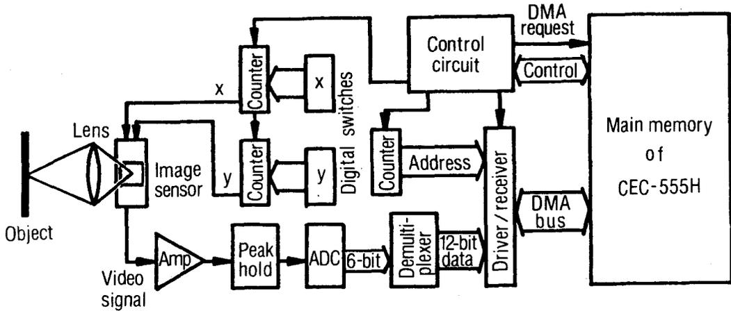
Fig. 6 Block diagram of the image-sensor input system.
