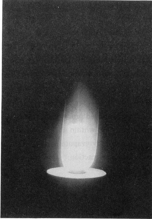
Fig. 2 Photograph of an ignited compact of a mixture of Ti and C powders.
