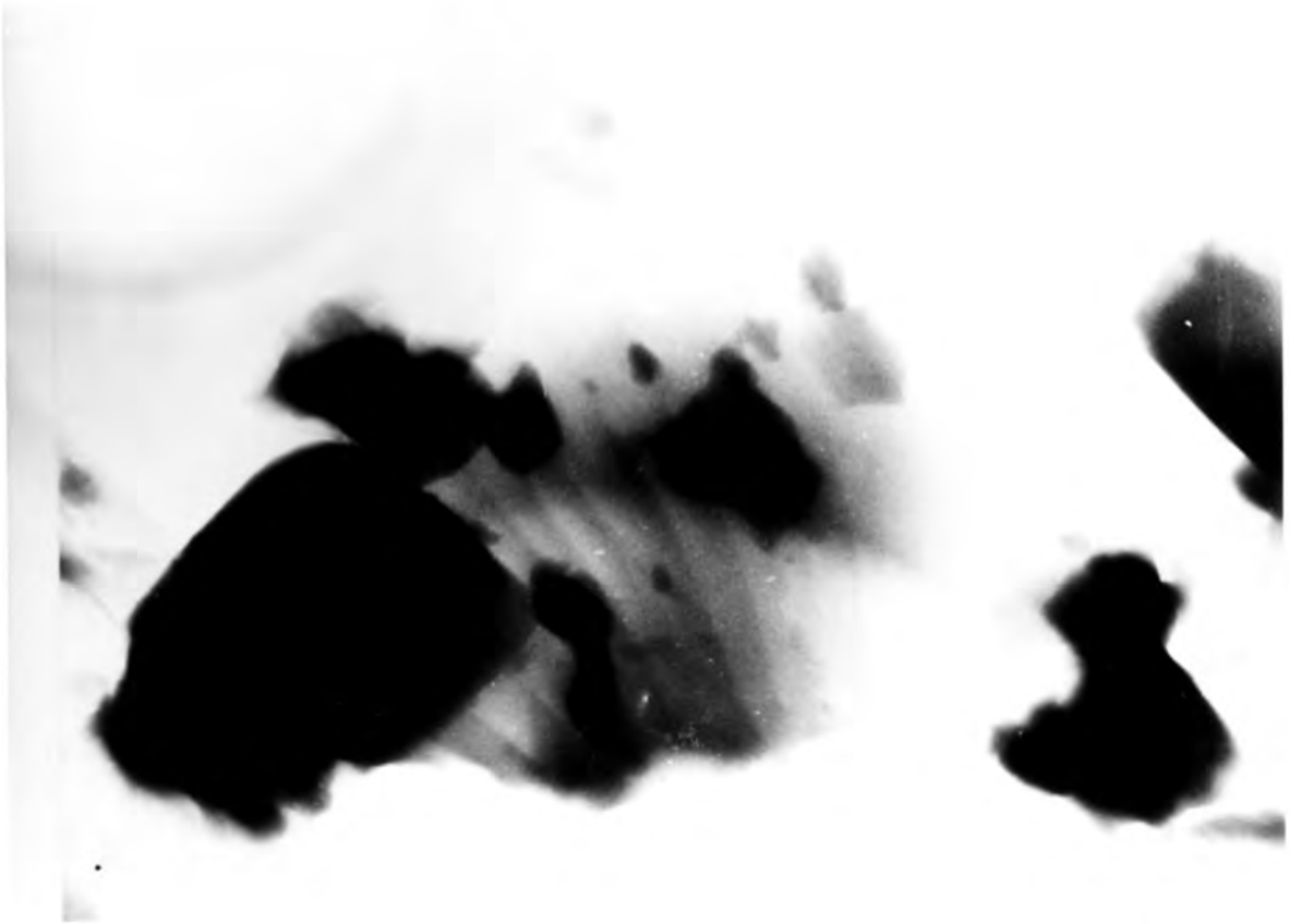
Fig.50 Homogeneous surface structure of fractured SiO 2 glass
