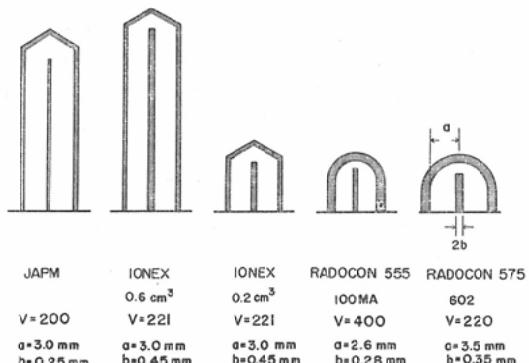
Fig. 1. Size and polarizing voltage of the chambers used.
