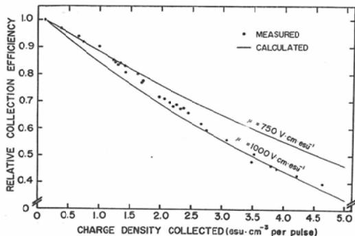
Fig. 2. Collection efficiency of an Ionex 0.6 cm<sup>3</sup> chamber plotted against charge density collected. Collection efficiencies were normalized to that for 0.1 esu·cm<sup>-3</sup> per pulse.
