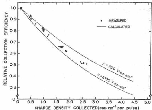
Fig. 5. Collection efficiency of a JAPM standard dosimeter plotted against charge density collected. Collection efficiencies were normalized to that for 0.1 esu·cm<sup>-3</sup> per pulse.
