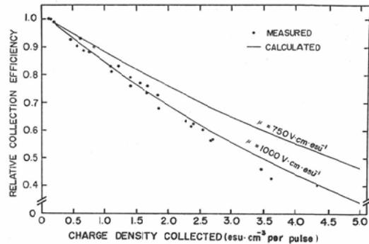
Fig. 3. Collection efficiency of an Ionex 0.2 cm<sup>3</sup> chamber plotted against charge density collected. Collection efficiencies were normalized to that for 0.1 esu·cm<sup>-3</sup> per pulse.
