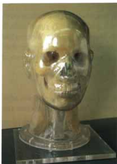
Fig. 7 Head phantom containing a human skull.
