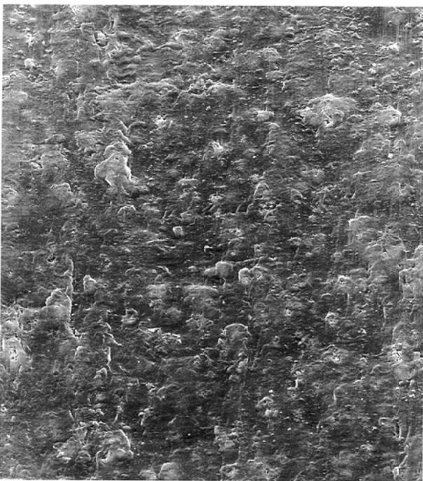
Fig.1 Scanning electron microscopic(SEM)image of the luminal surface of a catheter coated with FASUS copolymer. The surface shows lamellar microdomain appearance. ( $\times 3,600$ )
