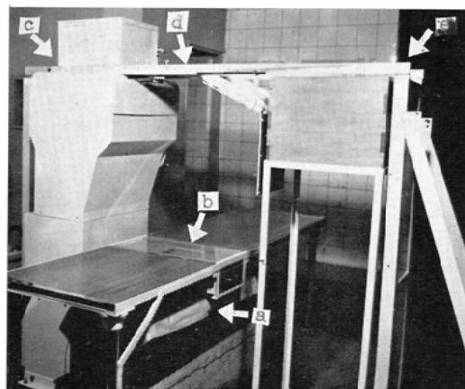
Fig. 6. Film cassette changer for enlargement angiography.
