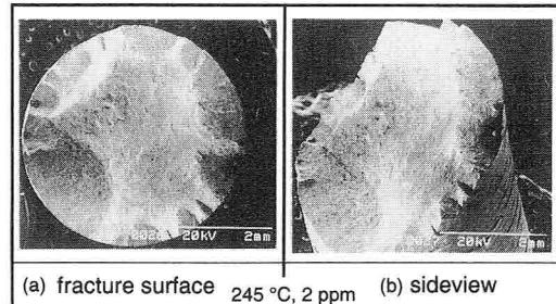
Fig. 5-2 The fracture surface of S45C-A specimen tested in 0.2 ppm O<sub>2</sub> water at 245 °C
