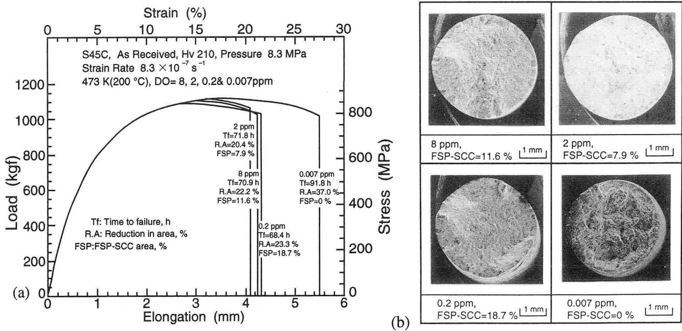
Fig. 2-11 S45C tested in 200 °C water at various DO environments.
