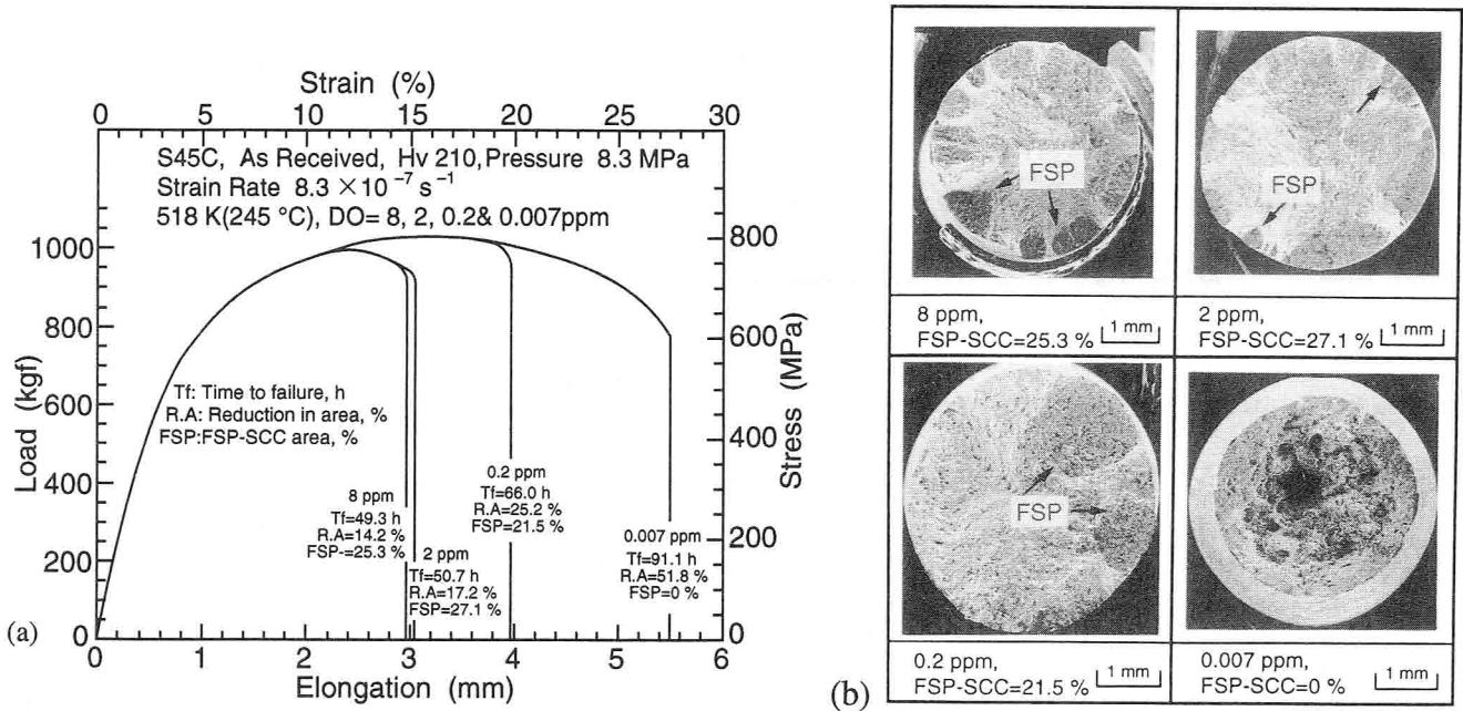
Fig. 2-12 S45C tested in 245 °C water at various DO environments.
