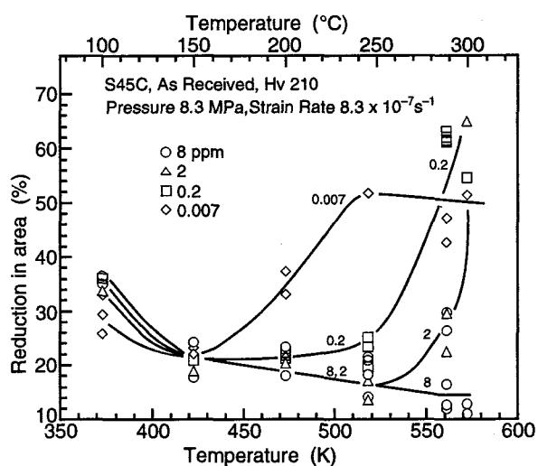
Fig. 2-16 Relation between reduction in area and temperature
