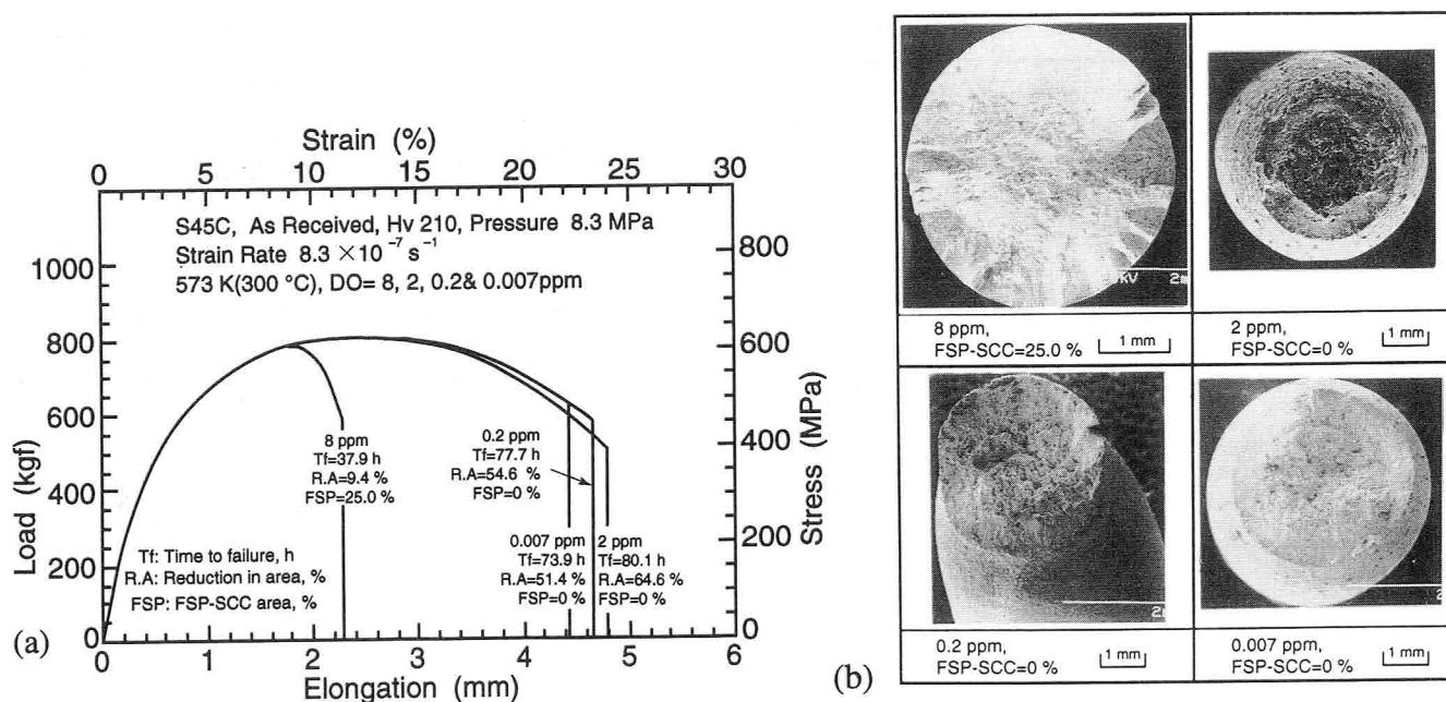
Fig. 2-14 S45C tested in 300 °C water at various DO environments.
