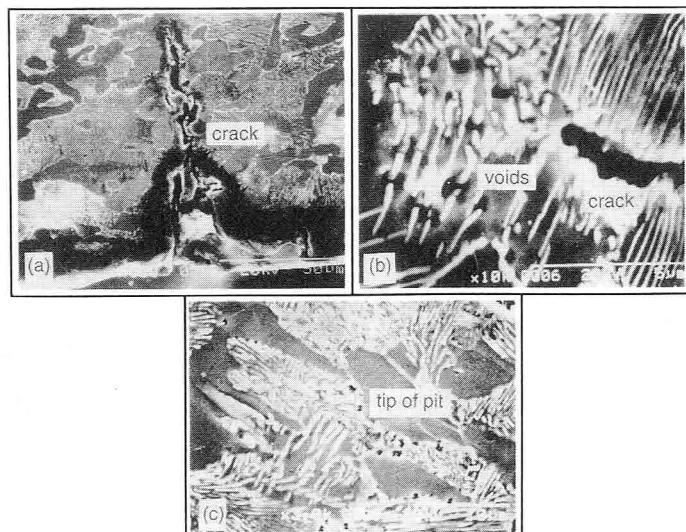
Fig. 5-8 Voids and microcrack in the pit
