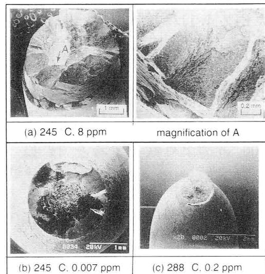
Fig. 4-9 The fracture surface of S45C quenched specimen tested in 8, 0.2 and 0.007 ppm O<sub>2</sub> water at 245 and 288 °C
