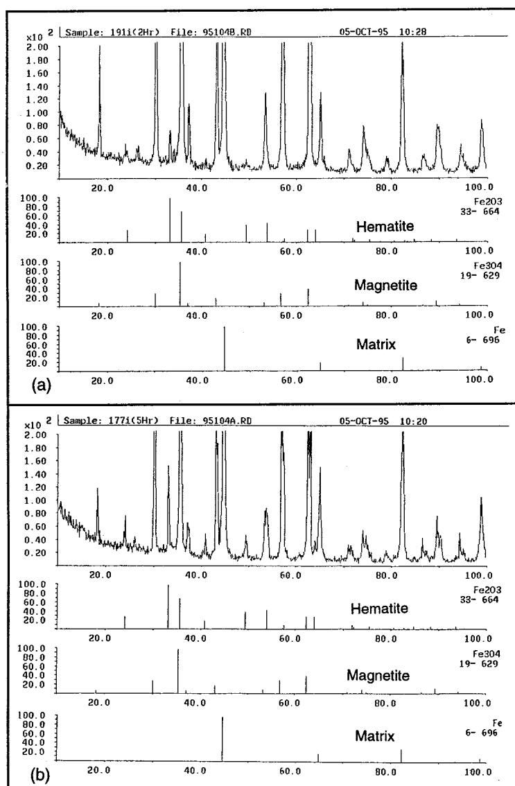
Fig. 5-17 Example of X-ray diffraction analysis tested in 8 ppm O<sub>2</sub> water at 245 °C
