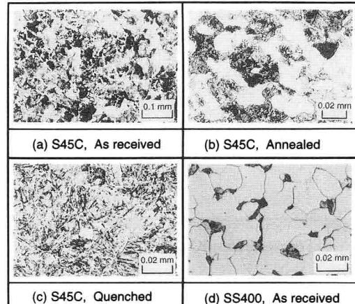
Fig. 4-1 Typical microstructures of steel tested
