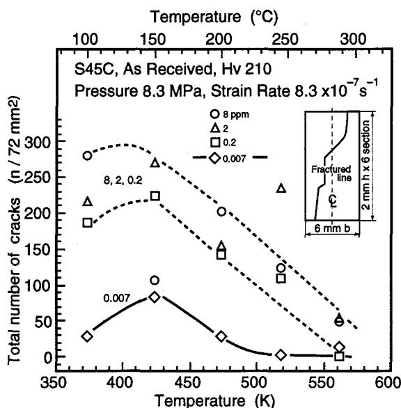
Fig. 2-19 The total number of cracks on the fractur side surface as a function of temperature at various dissolved oxygen
