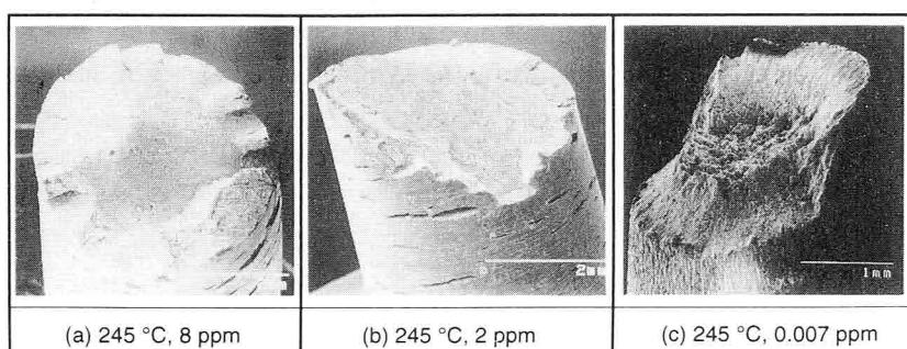
Fig. 4-15 The fracture surface of SS400 specimen tested in 8, 2 and 0.007 ppm O<sub>2</sub> water at 245 °C
