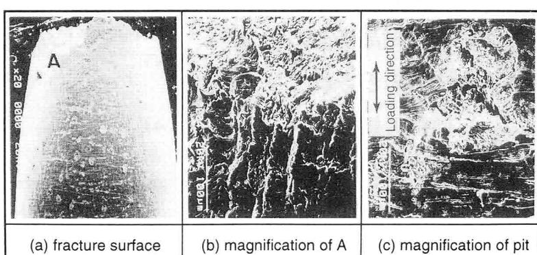
Fig. 5-16 The fracture surface of S45C-A specimen tested in 0.007 ppm O<sub>2</sub> water at 245 °C
