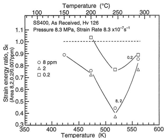
Fig. 4-13 Effect of dissolved oxygen on the strain energy ratio (SE: the ratio of the strain energy in 8, 2 and 0.2 ppm O<sub>2</sub> to that in 0.007 ppm O<sub>2</sub>)
