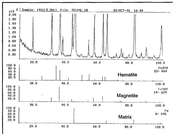
Fig. 5-18 Example of X-ray diffraction analysis tested in 0.007 ppm O<sub>2</sub> water at 245 °C
