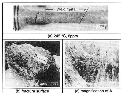
Fig. 4-19 The fracture surface of welded specimen tested in  $8 \text{ ppm O}_2$  water at  $245 \text{ }^{\circ}\text{C}$
