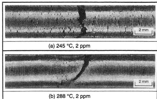
Fig. 2-20 The fractur side surfaces tested in 2 ppm O<sub>2</sub> (a) 245 °C, (b) 288 °C
