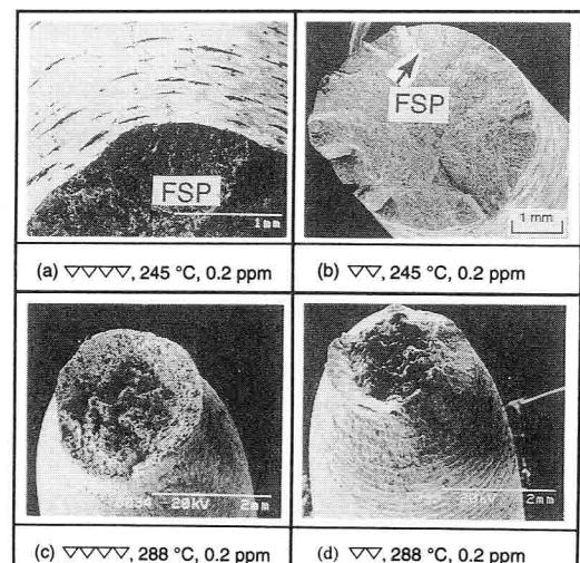
Fig. 2-5 The fracture surface of smooth and rough specimen tested in 0.2 ppm O<sub>2</sub> water at 245 and 288 °C
