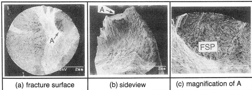
Fig. 2-3 Typical example of Fan-Shaped Pattern on the SEM photographs of S45C specimen tested in 8 ppm O<sub>2</sub> water at 245 °C
