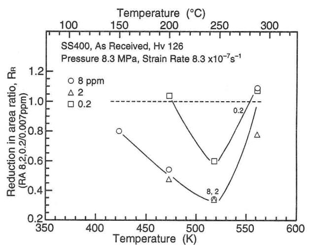
Fig. 4-14 Effect of dissolved oxygen on the reduction in area ratio (RR: the ratio of the reduction in area in 8, 2 and 0.2 ppm O<sub>2</sub> to that in 0.007 ppm O<sub>2</sub>)
