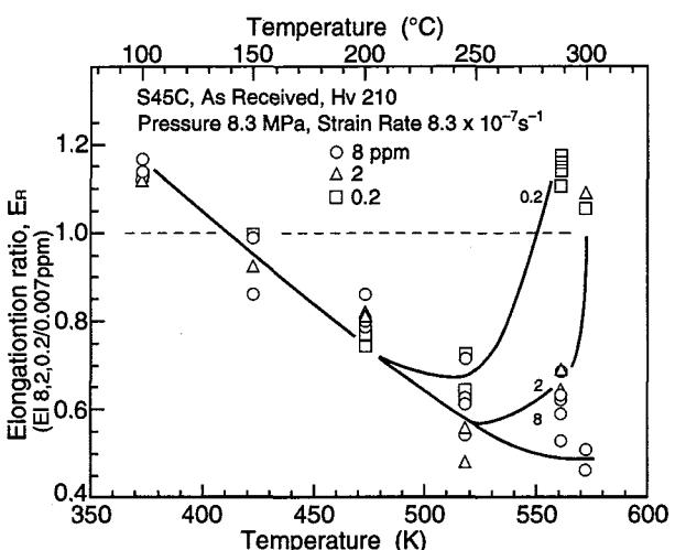
Fig. 3-2 Relation between elongation ratio and temperature (E<sub>R</sub>: the ratio of the elongation in 8, 2 and 0.2 ppm O<sub>2</sub> to that in 0.007 ppm O<sub>2</sub>)
