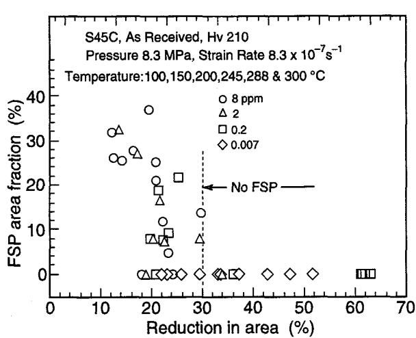
Fig. 3-5 Relation between FSP area fraction and reduction in area
