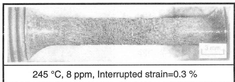
245 °C, 8 ppm, Interrupted strain=0.3 %
