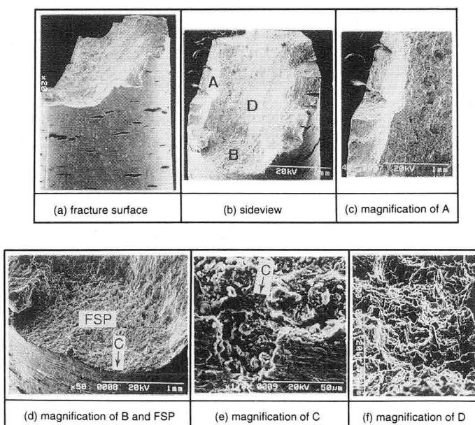
Fig.5-11 The fracture surface of S45C-A specimen tested in 8 ppm O<sub>2</sub> water at 245 °C
