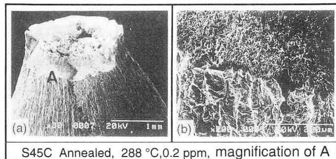
Fig. 4-6 SEM photographs of S45C annealed specimen tested in 0.2 ppm O<sub>2</sub> water at 288 °C
