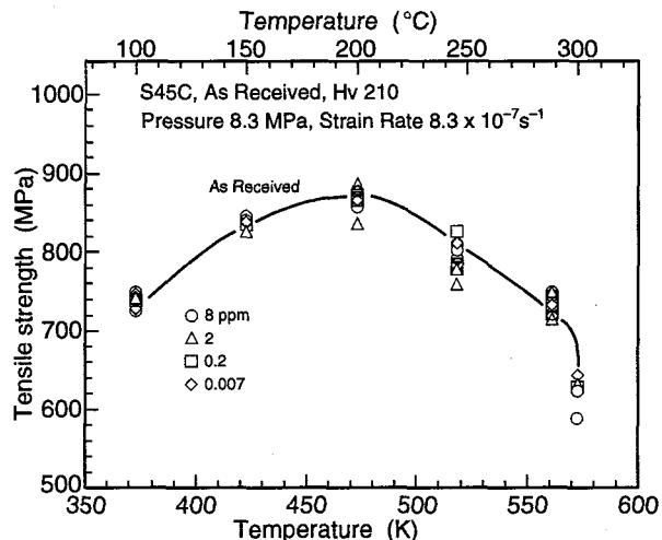
Fig. 2-17 Relation between tensile strength and temperature
