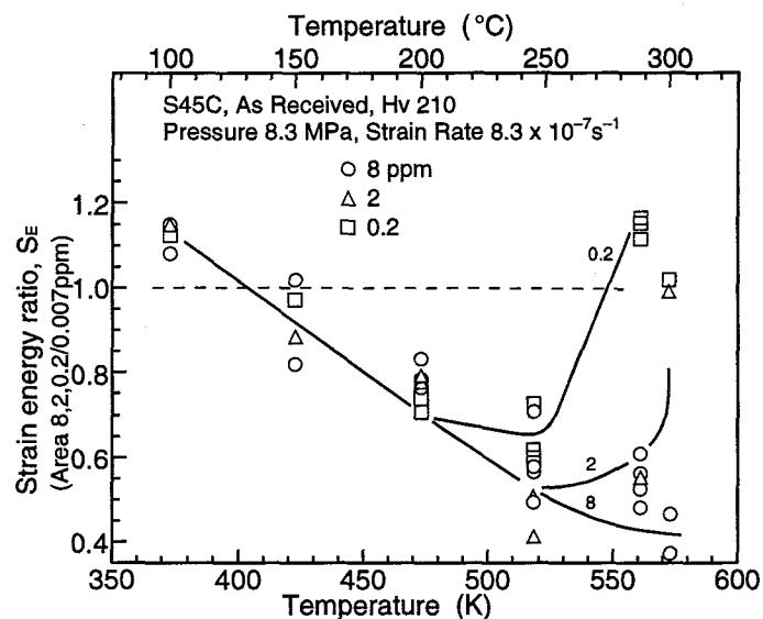
Fig. 3-4 Relation between strain energy ratio and temperature ( $S_E$ : the ratio of the strain energy in 8, 2 and 0.2 ppm O<sub>2</sub> to that in 0.007 ppm O<sub>2</sub>)
