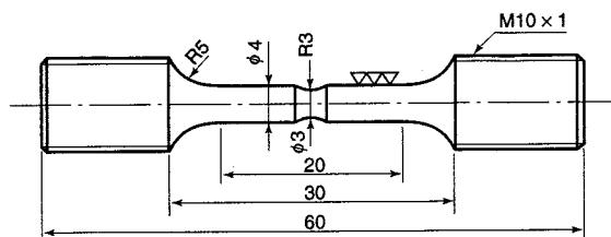
Fig. 4-20 Welded joint of the SSRT specimen
