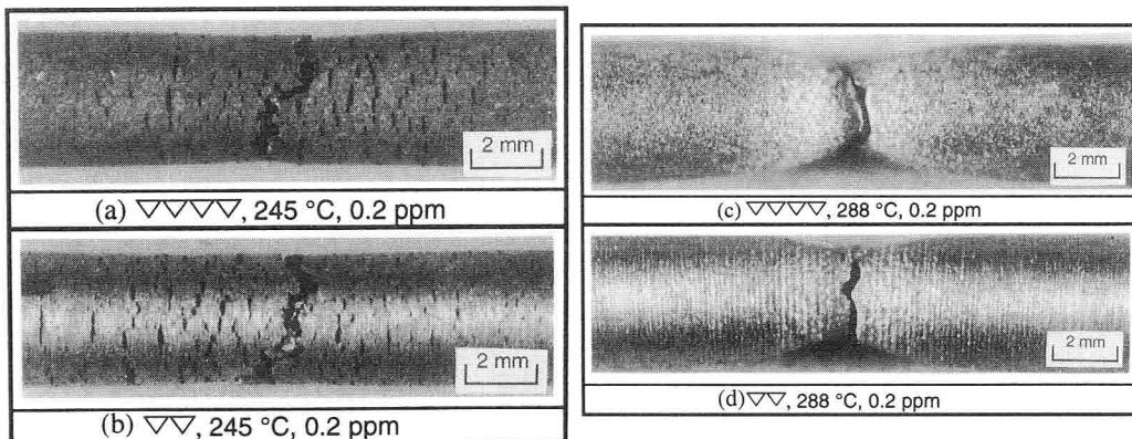
Fig. 2-6 The fractured side surface of smooth and rough specimen tested in 0.2 ppm O<sub>2</sub> water at 245 and 288 °C
