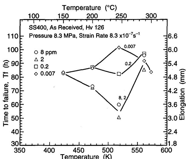
Fig. 4-12 Relation between time to failure and temperature
