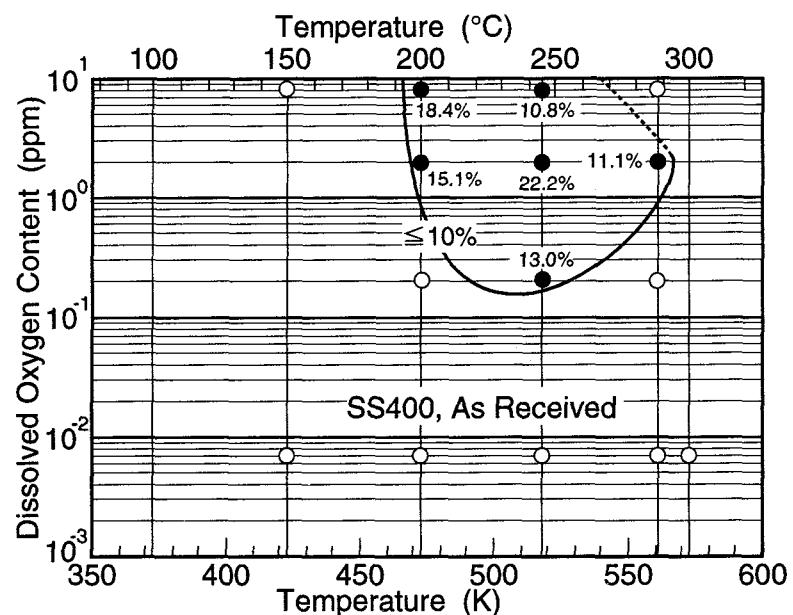
Fig. 4-17 Variation of the SCC ratio with oxygen and temperature
