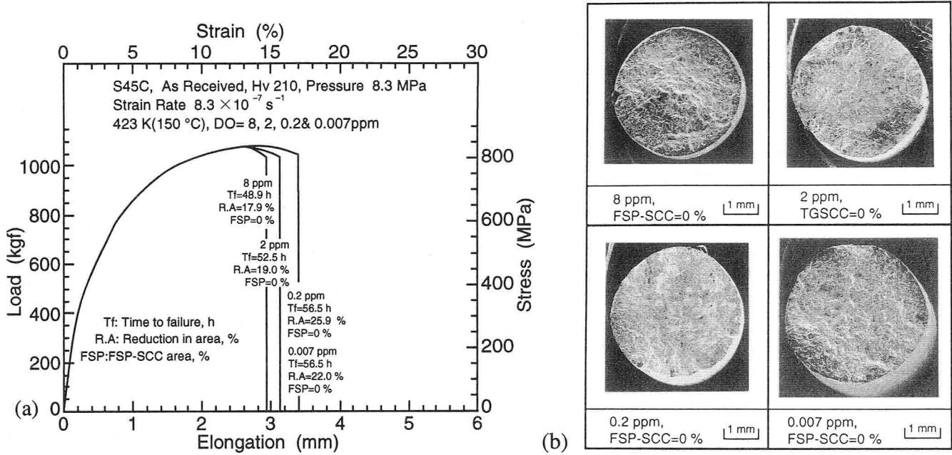
Fig. 2-10 S45C tested in 150 °C water at various DO environments.
