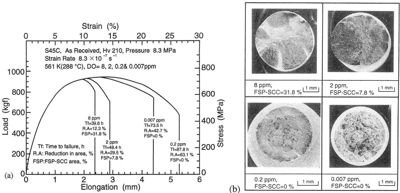
Fig. 2-13 S45C tested in 288 °C water at various DO environments.
