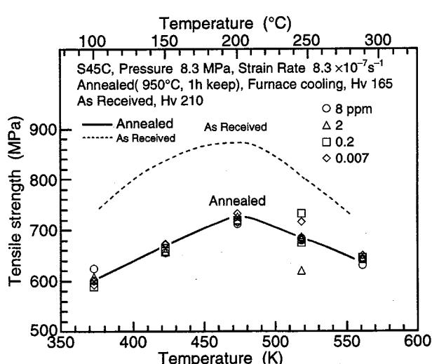
Fig. 4-2 Relation between tensile strength and temperature in annealed S45C
