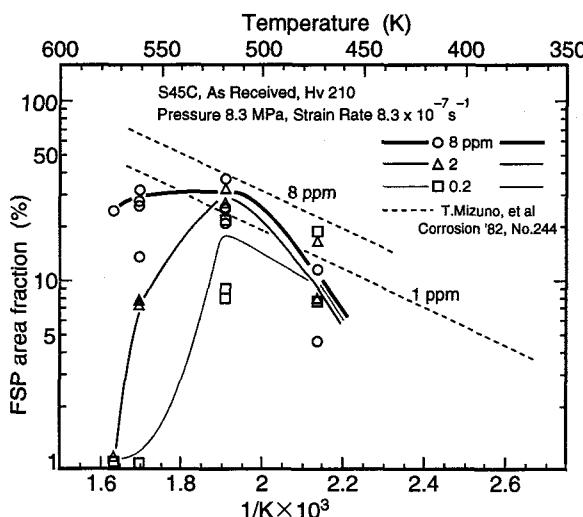
Fig. 3-6 Relation between FSP area fraction and temperature
