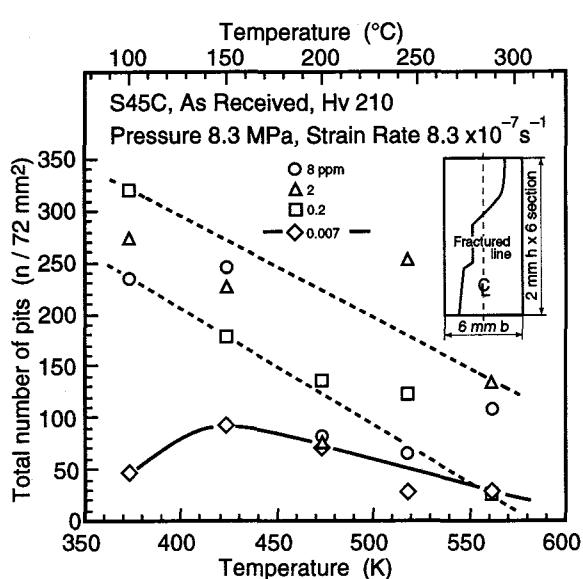
Fig. 2-18 The total number of pits on the fractur side surface as a function of temperature at various dissolved oxygen
