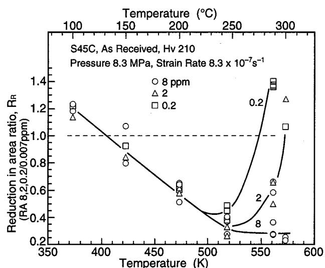
Fig. 3-3 Relation between reduction in area ratio and temperature ( $R_R$ : the ratio of the reduction in area in 8, 2 and 0.2 ppm O<sub>2</sub> to that in 0.007 ppm O<sub>2</sub>)
