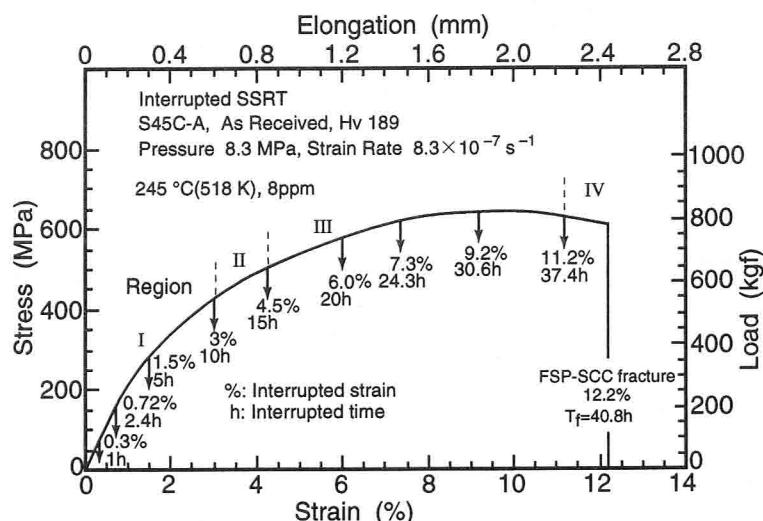
Fig. 5-3 Interrupted SSRT results
