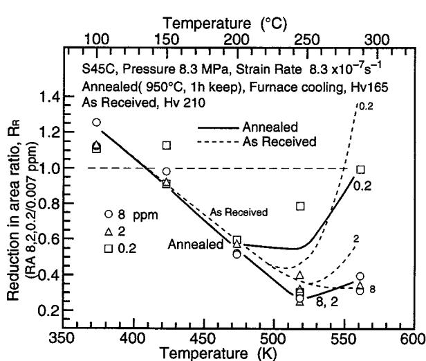
Fig. 4-4 Effect of dissolved oxygen on the reduction in area ratio ( $R_R$ : the ratio of the reduction in area in 8, 2 and 0.2 ppm  $O_2$  to that in 0.007 ppm  $O_2$ )
