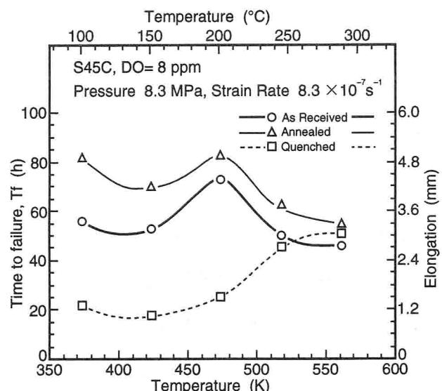
Fig. 4-10 Effect of S45C as received and heat treated specimen on the time to failure
