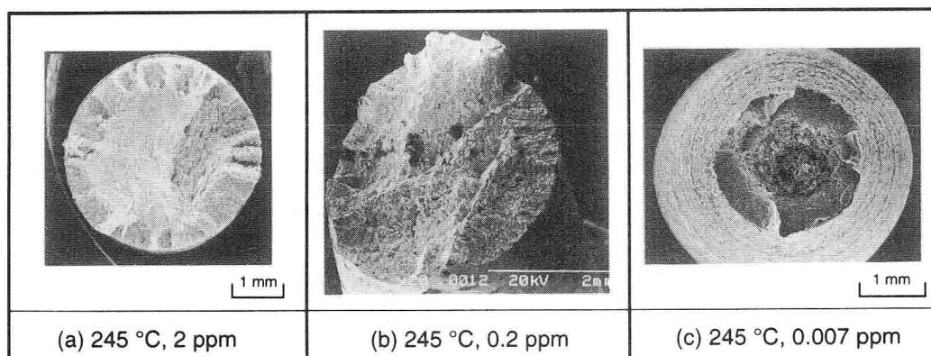
Fig. 4-7 The fracture surface of S45C annealed specimen tested in 2, 0.2 and 0.007 ppm O<sub>2</sub> water at 245 °C
