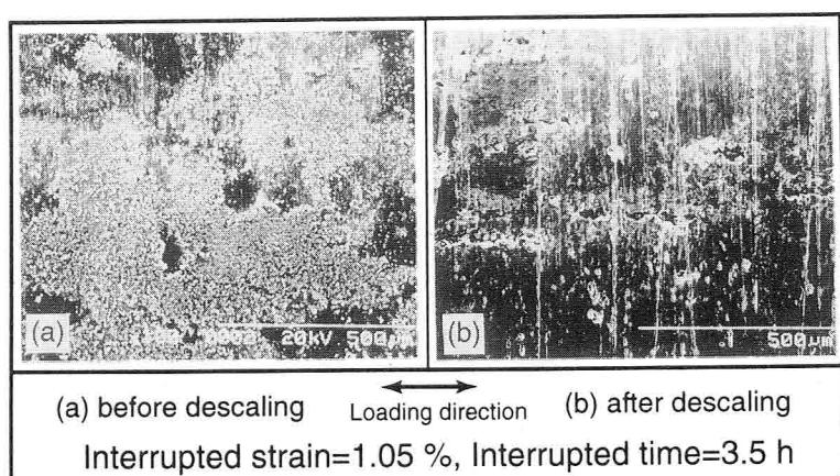
Fig. 5-14 SEM views of S45C-A interrupted specimen tested in 0.007 ppm O<sub>2</sub> water at 245 °C
