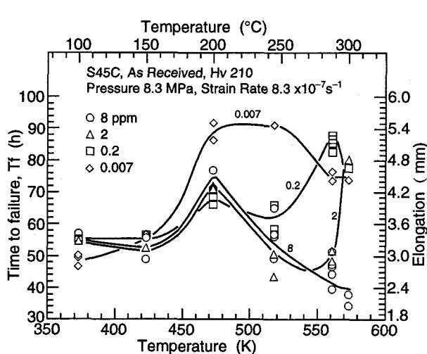
Fig. 2-15 Relation between time to failure and temperature
