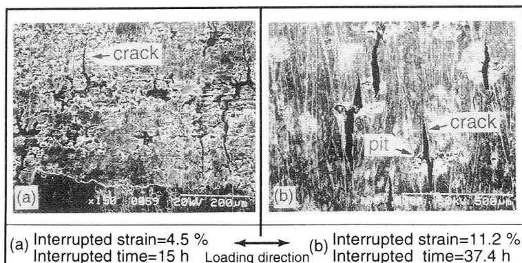
Fig. 5-9 SEM views of interrupted specimen after descaling tested in 8 ppm O<sub>2</sub> water at 245 °C
