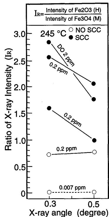
Fig. 5-20 Relation between ratio of X-ray intensity from two oxide layers and X-ray injection angle for the specimen tested in 245 °C
