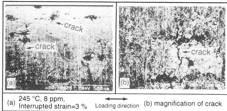
Fig. 5-7 SEM views of interrupted specimen after descaling
