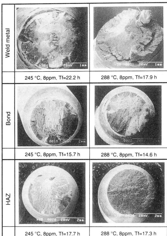
Fig. 4-23 Comparison among the fracture surfaces of different location of welded joint specimens tested in 8 ppm O<sub>2</sub> water at 245 and 288 °C
