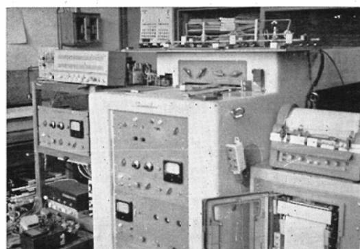
Fig. 2 The Scinti-Scanner With Multiscintigram System.
