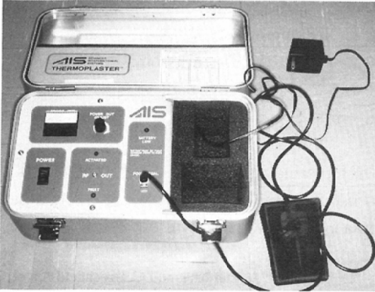
Fig. 1 Radiofrequency thermal angioplasty device. small-sized (41.2cm×23.5cm×14.8cm) and portable (6.8kg).
