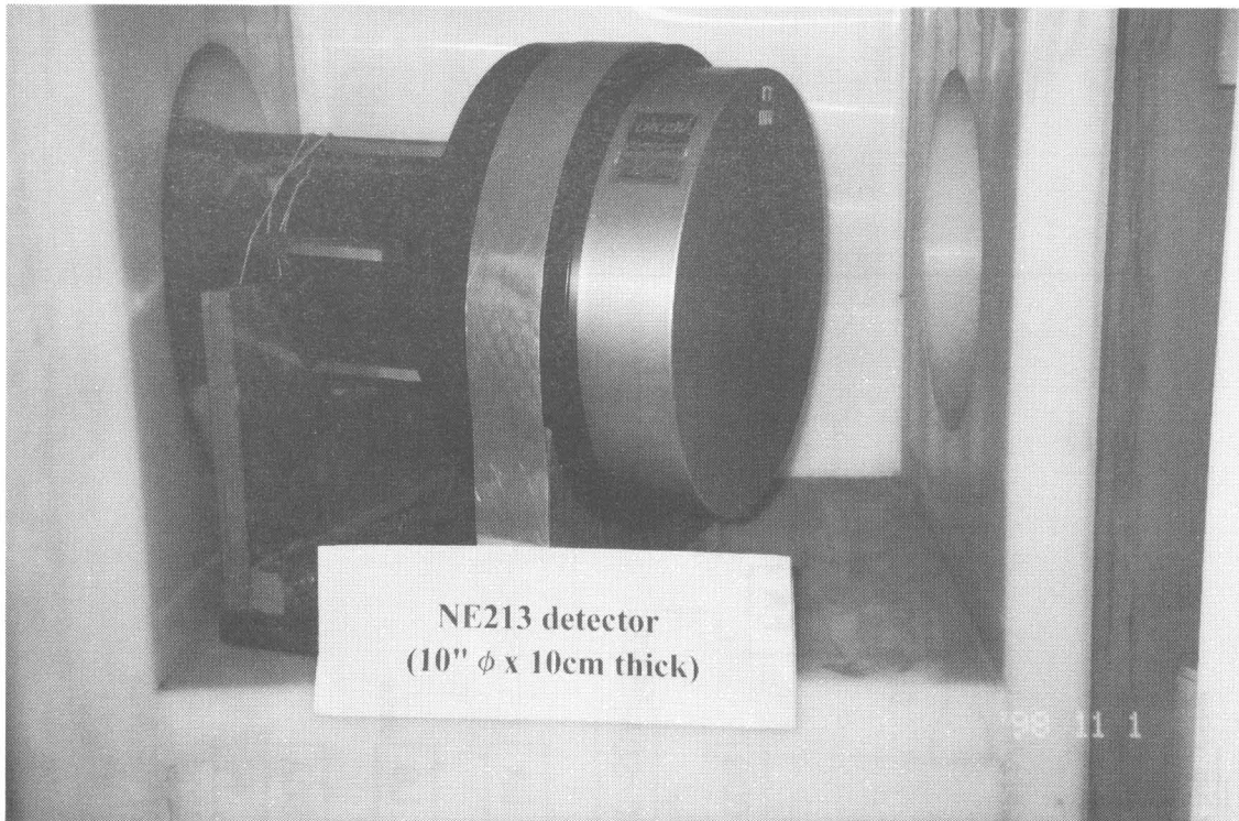
Fig. 4.16 Large NE213 detector (10" \phi x 10 cm) used to measure high energy neutron spectrum with TOF method in the present experiment.
