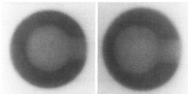
Fig. 3 Verification films were taken to evaluate geometric and mechanical accuracy in various combination of gantry and table angles. There was no error at the position of gantry angle 0° and table angle 0° (Left). Maximum error was observed at gantry angle 90° and table angle 45° (Right).
