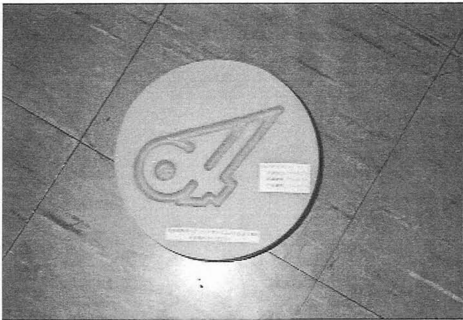
Fig. 6-17 Machining Experiment, Result of the Character Line Milling
