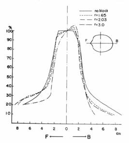
Fig. 5 Dose distribution in the hollow-out technique applied to 6 Mev linear accelerator. The longer the radius of protected area, the larger the deviation of isodose contour. Field size is 4cm ×4cm.
