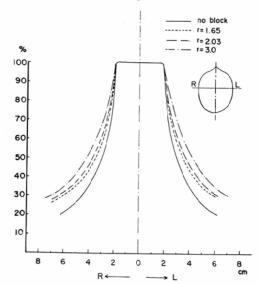
Fig. 4 Relative dose distribution along the long axis of phantom in selective protection technique of the eye balls with 6 Mev linar accelerator.
