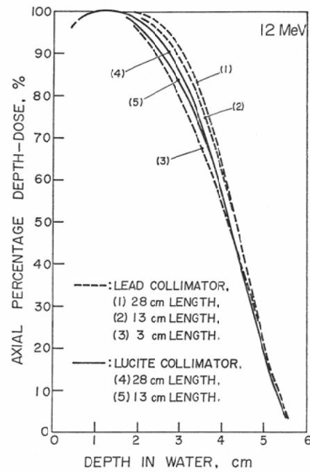
Fig. 9a. Central axis percentage depth dose in water for  $6 \times 6$  cm field, and for 12 MeV.
