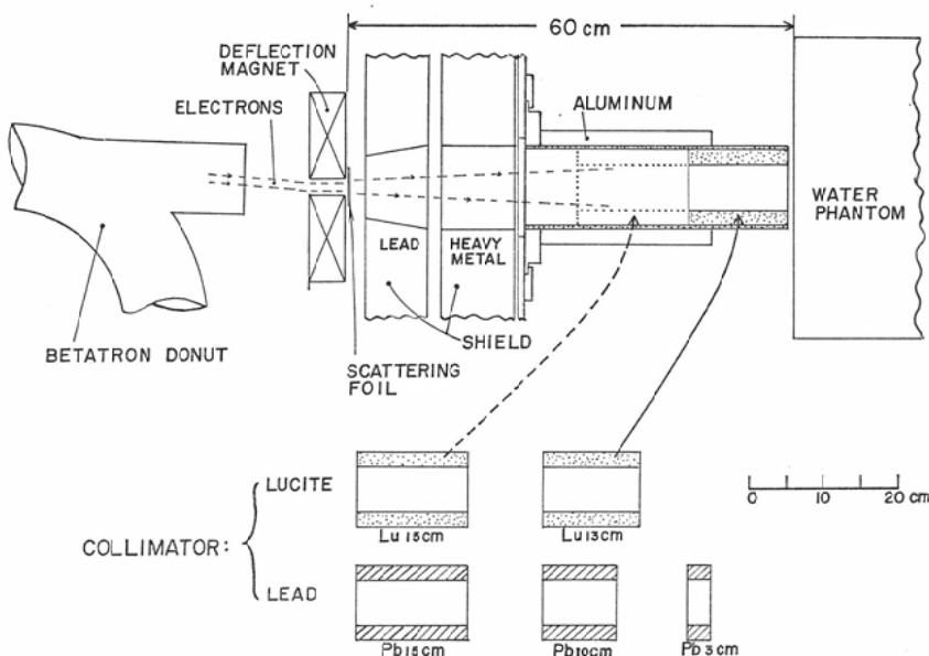
Fig. 6. Schematic diagram of the collimation system for 6×6 cm field. The distance between the scattering foil and the phantom is 60 cm (fixed). The collimator length is defined as below: if only Lu 13 cm collimator is used, the length is 13 cm; if both Lu 13 cm and Lu 15 cm ones are used, the length is 28 cm; and so on.
