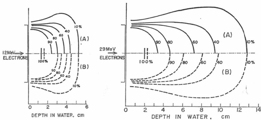
Fig. 8. Isodose curves within water for 12 MeV and 29 MeV electrons, for  $6 \times 6$  cm field. Curves are given for lead collimators of 3 cm (A) and 28 cm (B) length.
