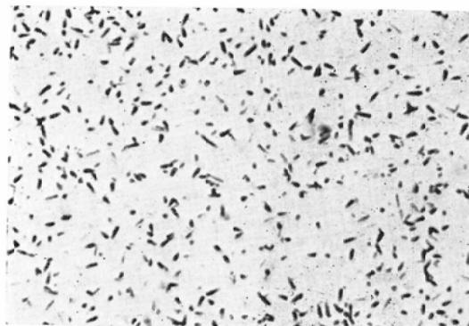
Fig. 3. The etched pits in the plastic film.
